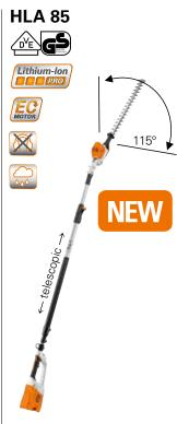
The cordless hedge trimmer for professional applications, with a telescopic shaft that provides long reach. Infinitely variable speed control, adjustable for vertical, overhead and ground-level cutting, cutter bar adjustable by 115°, double-sided cutting blades. Tool-free adjustment of the shaft length using quicktensioning lever, transport length of 180 cm, total length of 260-330 cm. Weight 4.4 kg<sup>3</sup>. For more information on the features and technical details, see page 129.
