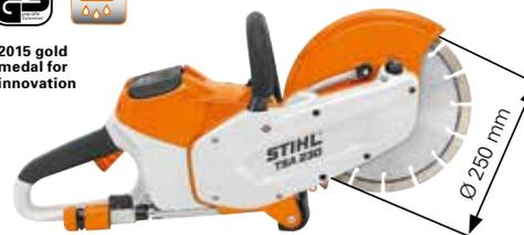
Easy-to-manoeuvre battery cut-off machine for 230 mm cutting wheels. Suitable for indoor and outdoor use, up to 70 mm cutting depth, water connection with ball valve and hose coupling for wet cutting, spindle lock, maintenance-free belt drive. Weight: 3.9 kg <sup>Ⓣ</sup>.
