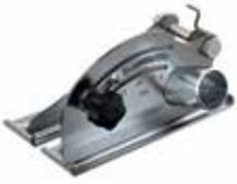
The depth stop with vacuum support enables dust-free cutting of mineral construction materials on flat surfaces. Exact and continuously adjustable cutting depth possible for TSA 230.
