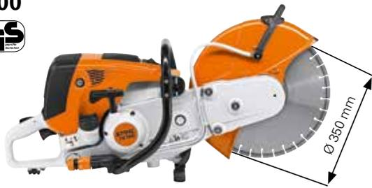
**98.5 cm<sup>3</sup>, 5.0 kW/6.8 hp, 11.7 kg<sup>①</sup>**. Most powerful cut-off machine for 350 mm cutting wheels. The cut-off machine is perfectly suited to use at full cutting depth and also on the FW 20 cart. Equipped with decompression valve and STIHL ElastoStart for effortless starting and the long-life air filter system. Economical 2-MIX engine.
