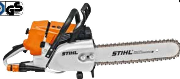
**76.5 cm<sup>3</sup>, 4.3 kW/5.8 hp, 7.6 kg<sup>①</sup>.** Handles like a chainsaw, with the power of a cut-off machine. Side-mounted chain tensioning, STIHL anti-vibration system, water connection, decompression valve, STIHL ElastoStart, wear-resistant starter cord, HD2 filter, tank with bayonet fuel cap for upright refuelling, 2-MIX engine.
