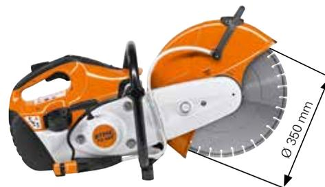
**66.7 cm<sup>3</sup>, 3.2 kW/4.4 hp, 9.7 kg<sup>Ⓞ</sup>**. An all-purpose cut-off machine for above and below ground. With 350 mm cutting wheels to cut up to 125 mm deep. The STIHL anti-vibration system guarantees the cut-off machine cuts well. Long-life air filter system, strength-saving start-up process thanks to the decompression valve, economical 2-MIX engine.
