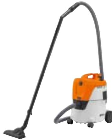
**1.4 kW, 210 mbar, 3,600 l/min.** For getting rid of dust, dirt and liquids indoors and outdoors. Wet and dry vacuuming options, blower function by moving the suction tube to the exhaust port, multiple filter system, filter cleaning, switchable floor nozzle, universal nozzle, crevice nozzle.
