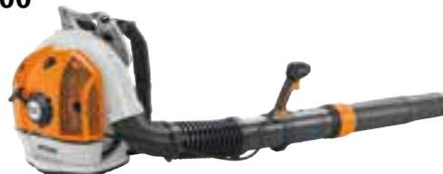
**64.8 cm<sup>3</sup>, 10.8 kg<sup>Ⓞ</sup>**. The ultimate high-performance blower with outstanding blowing power. Tool-free adjustment of the handle position and adjustment of the blower tube length. Soft handle. STIHL anti-vibration system, 4-MIX<sup>®</sup> engine. Ergonomically shaped, wide shoulder straps, hip belt, locking throttle lever with stop button, carry handle. The optional bike handle (4282 790 1700) is recommended when working with curved nozzles for long periods.
