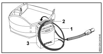
The length of the connecting cable can be adjusted by making a loop (1) and securing it to the belt bag (3) with the fastener (2).
