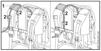
The connecting cable can be secured in position by the guide (1) on the harness and the fasteners (2), or on the side of the backplate with the fasteners (2).
