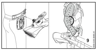
Attach the blower to the deluxe carrying system. The height of the plate (8) is correct when the user's arm is slightly bent while holding the front grip (9) to control the blower.
